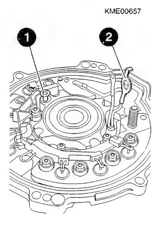
DISMANTLING AND CHECKING ALTERNATOR Dismantling pole body Detach drive-end shield (1) from pole body (2). Pay attention to connections (3) and (4).
